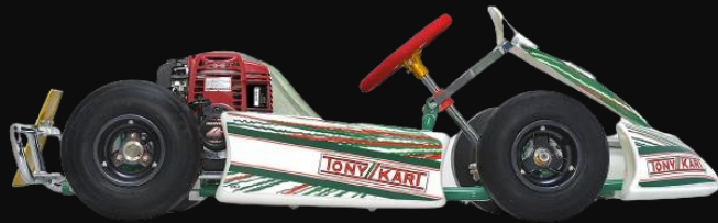
Kid Kart Chassis ~770-900mm Wheelbase
