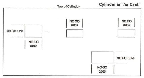
Aluminum Cylinder "As Cast". Engine is not legal if any metal has been removed to match port opening to aluminum cylinder.
