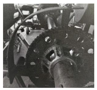
**2-cycle:** All chain, belt or gear-driven karts must be equipped with a chain, belt or gear guard designed to retain a broken chain, belt or gear. Karts with outboard drive systems, must have a guard or third bearing support on the engine. Kart must also have a rear sprocket guard. Rear guard must cover 25% or rear sprocket and be a minimum of 1.5" wide.
