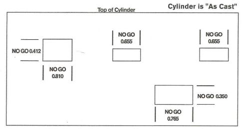
Aluminum Cylinder "As Cast". Engine is not legal if any metal has been removed to match port opening to aluminum cylinder.
